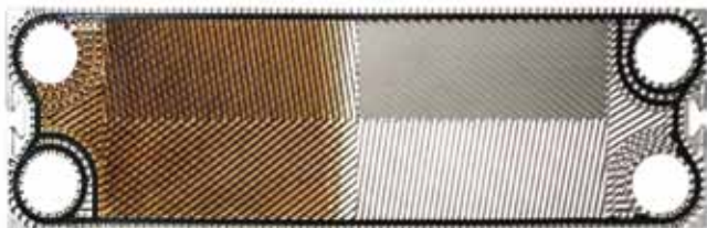
Dirty plates effect heat transfer and reduce the overall performance.
