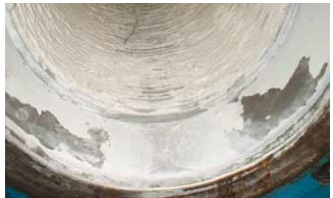
These are the conditions in which you could find your plate heat exchanger without regular maintenance.
