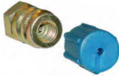
MT0141 QTY: 5 R134a Retro Fitting Low Side Steel w/ Schrader Line Thread: 7/16"-20 Female Cap Thread: M13-1.0 Female w/ Schrader Cap: MT0063
