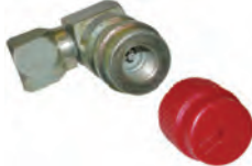
MT0148 QTY: 1 R134a Retro Fitting 90 Degree Swivel w/Cap- High Side Line Thread: 7/16"-20 Female Cap Thread: M15-1.0 Female w/ Schrader Cap: MT0069
