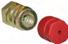
MT0143 QTY: 5 R134a Retro Fitting High Side Steel w/ Schrader Line Thread: 7/16"-20 Female Cap Thread: M15-1.0 Female w/ Schrader Cap: MT0069
