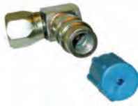
MT0147 QTY: 1 R134a Retro Fitting 90 Degree Swivel w/Cap- Low Side Line Thread: 7/16"-20 Female Cap Thread: M13-1.0 Female w/ Schrader Cap: MT0063
