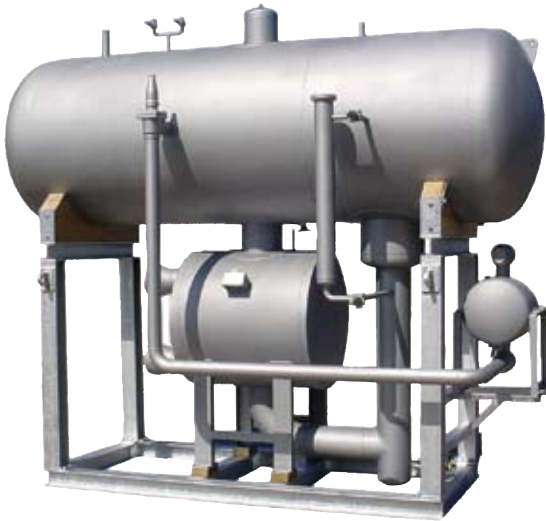
Two SPW-55 R507 evaporators in parallel with separator. Skid for a Climate Testing Laboratory supplied to the Automotive Industry.
