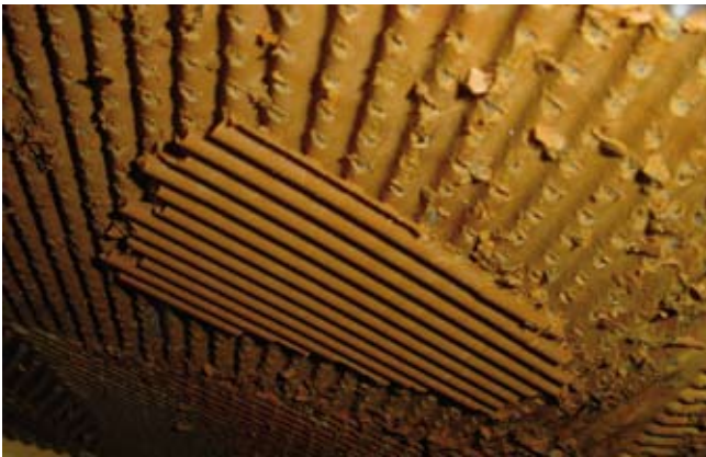
Pollution increases the pressure drop and your energy costs. It can also damage the plates or the gaskets.
