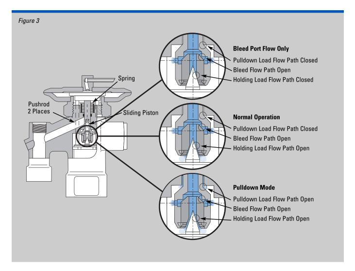
The addition of a resealable bleed port allows for more stable superheat control with medium temperature applications. Figure 3 shows the bleed port which opens as the valve begins to operate. As the stroke of the bleed port is reached, the small capacity port begins to open. At this point, the valve regulates in the same manner as a conventional TEV. During pulldown, all three ports will be open.
