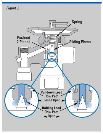
the coil during pulldown. But the more oversized the valve, the less capable it is in maintaining stable superheat at low load conditions, particularly when variations in condensing pressure from summertime to wintertime operation are considered.
