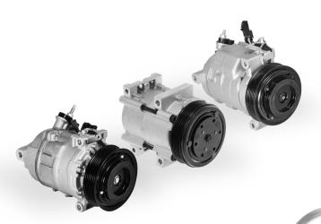
The compressor is responsible for pressurizing and circulating the refrigerant gas, enabling it to absorb heat from the vehicle's interior, and then compressing it into a high-pressure, high-temperature gas before it enters the condenser for heat dissipation.
